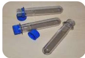
Tube after processing at factories, used to make bottles
